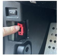
Place the inner part of the OBD lock on top and over the narrow side of the trapezoidal OBDII port. You may need to keep a finger on it to hold in place.
