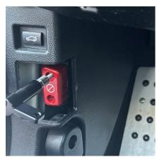
Using the provided VTT tool, fully install the proprietary Anti-Tamper Screws hand tight. Note that the screws bite into the sides of the unused center section of the OBDII port, so there is no concern of damaging electrical pins.
