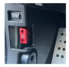
While keeping the inner part of the OBD lock in place, slide the outer shell over the entire assembly. Note this may be a tight fit, but should not require excessive force to push in place.
