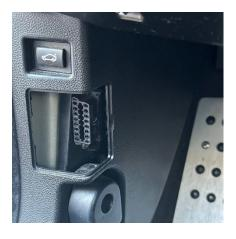
Locate your vehicle's OBDII Port and remove access cover
