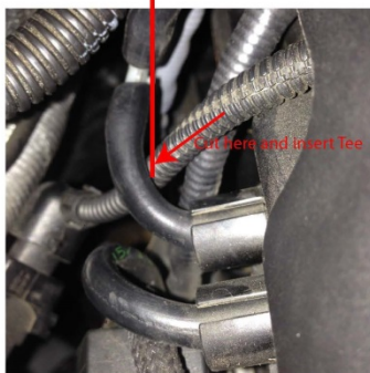
Vacuum source from valve cover
